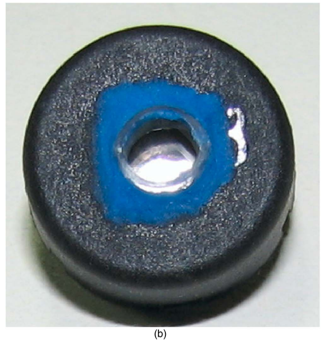
FIG. 13. (Color online) The piezoelectric buzzer with a duct resulting from the design chart method. (a) Cross-sectional diagram and (b) photo of the mockup.
