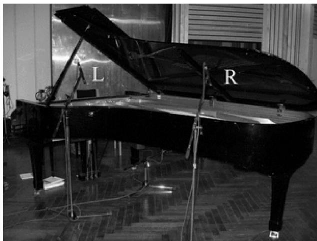
FIG. 1. Illustration of the microphone positioning above the string register. The letters L and R indicate the locations of the microphones corresponding to the left and right channel, respectively.
