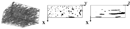
FIG. 1. Three-dimensional porous network (pores are in grey) in a parallel-epipedic block extracted from the \mu CT reconstructed bone structure. On the right-hand side are shown a transverse and longitudinal cross section through the three-dimensional porous network. The preferential orientation of the pores is along the bone axis.
